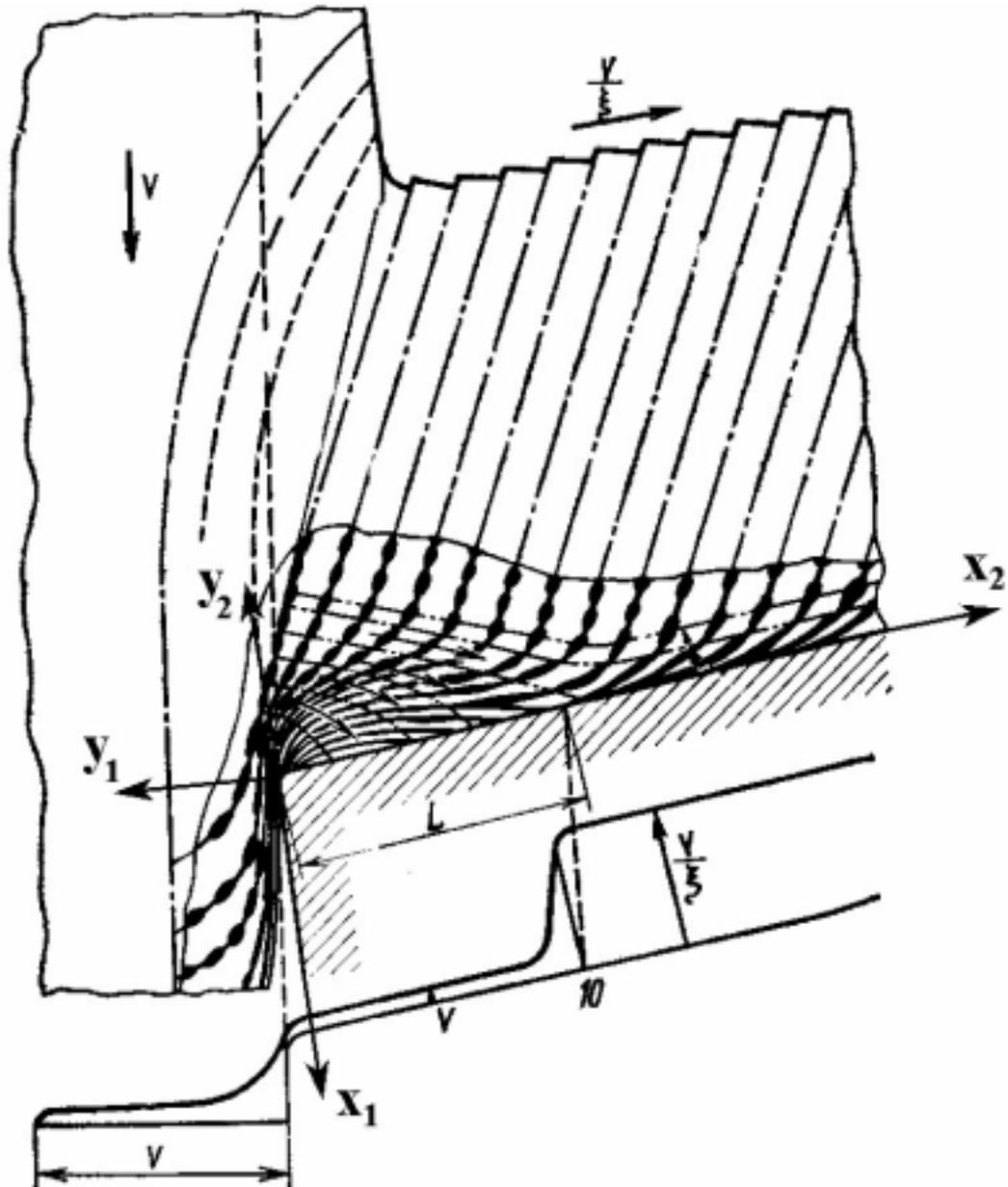
Fig. 2.1. The flow's scheme of layer to be cut and work surface.
