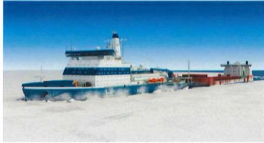
Universal atomic icebreaker Project 22220 (IB60) with the propulsion power of 60 MW
