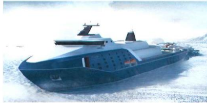
Atomic turbo-electric icebreaker Project 105010 (IB Leader) with the propulsion power of 120 MW
